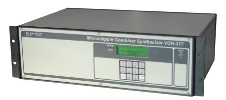
Microstepper Combiner Synthesizer VCH-317, produces an uninterrupted in frequency and phase signal on the base of group atomic clocks. Operational principle of Combiner is based on frequency control of local crystal oscillator using multichannel phase comparator and digital processor. Digital control of output frequency performed by built-in processor provides such advantages as programming frequency and phase shifts of output signal with high resolution.
