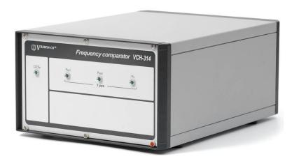
Frequency comparator VCH-314 is intended for precise phase and frequency measurements of three signals from frequency and time standards. Comparator contains two identical measuring channels and perform synchronic measurements of input signals phase difference. Using a correlation computing of measuring data, comparator precisely calculates frequency and phase difference between input signals and frequency instability for each signal separately.
