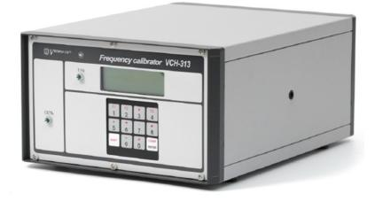
Frequency calibrator VCH-313 is intended for calibration and verification of different frequency signal sources, using precision time scale signal, transmitted by satellite navigation systems GPS/GLONASS. The instrument can provides periodical frequency correction of the calibrating frequency standard in automatic mode.
