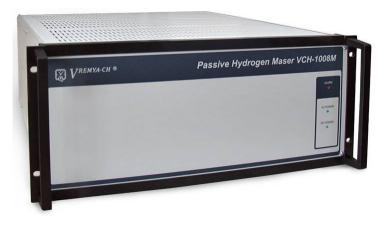
VCH-1008M Passive Hydrogen Maser is a compact hydrogen maser with excellent frequency stability and utilizes state-of-the-art technology. Full digital processing of the modulation and servo loop signals makes it ideal for high accuracy applications. An internal GPS/GLONASS option is available and provides automatic output signal frequency calibration. The device is remotely control via RS-232C, USB or LAN interfaces.
